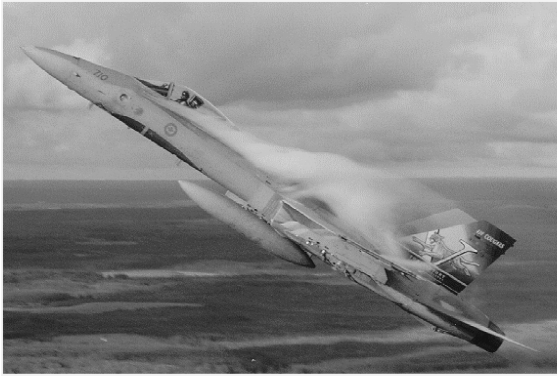
Fig. 1 Vortices breakdown upstream of the vertical fin.
